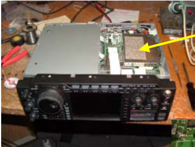
Picture 1. DSP unit. Unplug and set aside.
