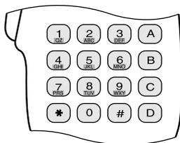
You can also use the Mic keypad to program a memory channel name {pages 36 and 58}, Power-on message {page 68}, or other character strings. Each press of a Mic key switches entry of characters as below. You can always use Mic **[A]** as **[➡]**, **[B]** as **[⬅]**, **[C]** as **[DEL]**, and **[D]** as **[OK]**.
