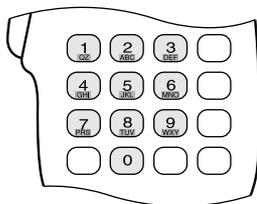
To manually send a DTMF number, press and hold Mic **[PTT]**, then press the DTMF keys on the Mic keypad {page 57} in sequence.
