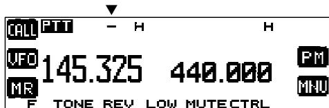
If the offset transmission frequency falls outside the allowable range, transmission is inhibited. Use one of the following methods to bring the transmission frequency within the band limits:
