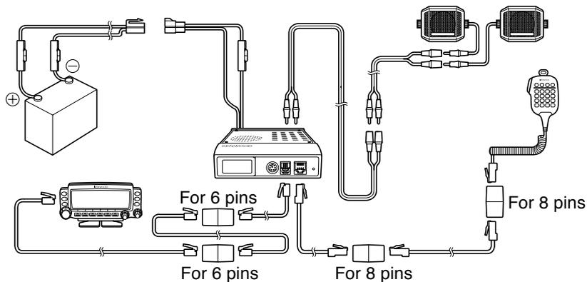
**Note:** Always connect the 4-pin plug on the modular plug cable supplied with the transceiver to the front panel.
