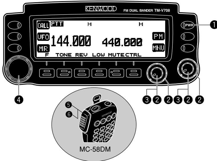
**1** Switch the DC power supply ON, then press the **PWR** switch.
